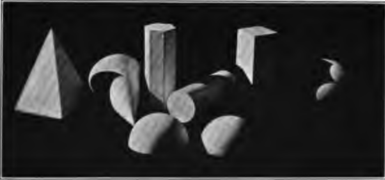
Fig. 20 — Illuminated by a point source at the left forty-five degrees above the plane. Illustrates the influence of the shape of the receiving surface on the appearance of the shadow.
